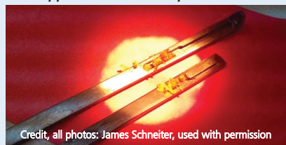
Above and below: Cutaway of a laparoscopic instrument showing bioburden trapped inside of the square corners
